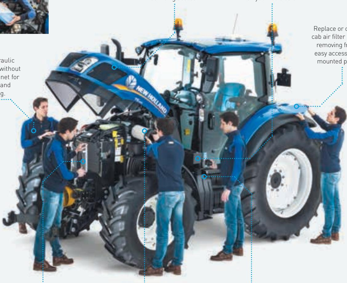
Replace or clean the cab air filter by simply removing from the easy access fender-mounted position.
