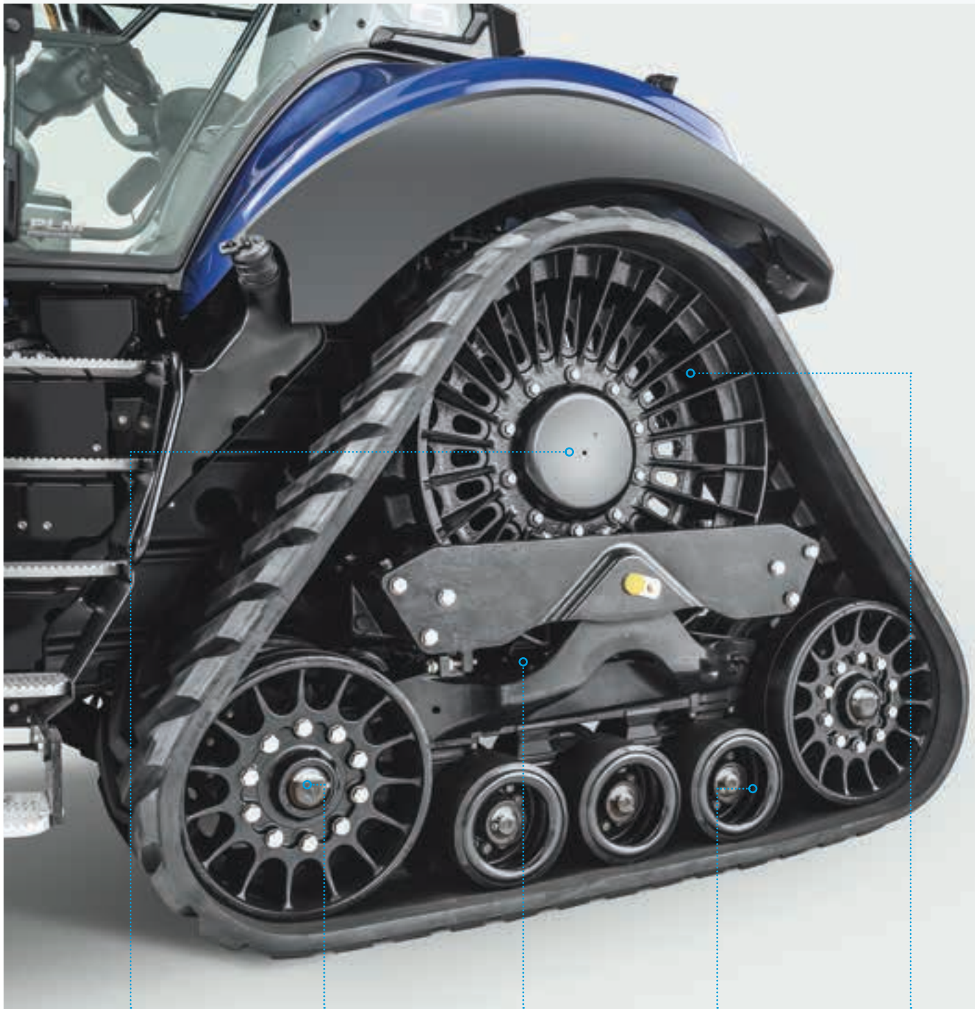
Ductile cast iron drive wheel
