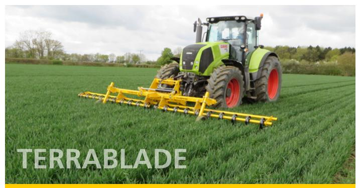
Experience has shown that the TerraBlade can be driven at speeds between 8-12km/h. It can be used quite late in the spring in favourable conditions, even when the crop is at growth stage 32.
