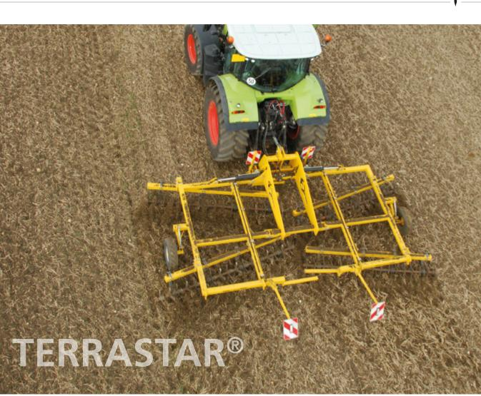
If there are very high levels of crop residue, or manure is spread on the field, then the TerraStar<sup>®</sup> offers a solution without destroying the soil profile. It will cultivate deeper than the straw harrow leaving divots in the soil. The design of this two rotor machine cultivates just enough to incorporate residue into the soil whilst leaving soil structure undamaged. The divots in the soil created by the TerraStar<sup>®</sup> also inhibit erosion, particularly on hillsides.
