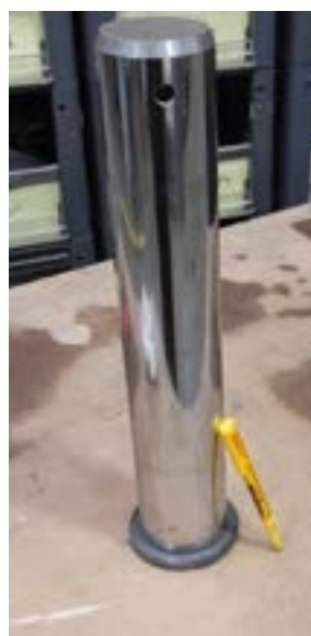
Robust wing pivot pin (440mm long, 80mm diameter)
